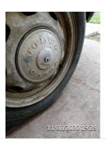
Wheel hubs and the centre bolts. I have all 4. One has the bolt missing, two have heavy dents. Worst case I just need a bolt.
